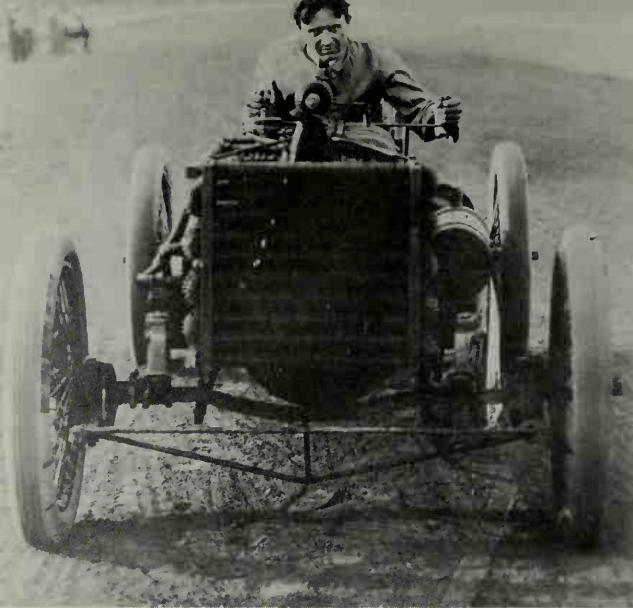
A head-on view of 999 showing the modified finned-tube radiator.
